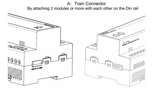
B- Screw terminals connection By using the Cat5e cable to connect to TIS bus 4 terminals (24V,D+, D-, GND)
