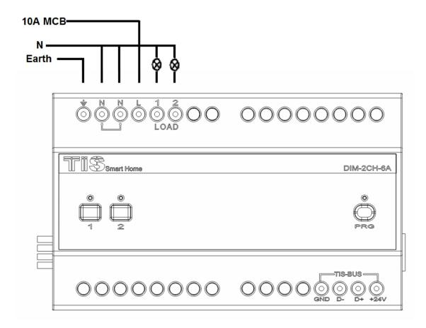
Nutral /Phase connection (N/L): Load connection (1,2) : Earth connection: 4 mm electrical wire2.5 mm electrical wire.2 electrical wire.
