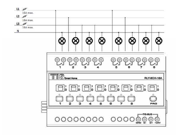
Input Phase: Load connection (1,2,3,4) : 1.5 or 2.5 mm electrical wire. 1.5 or 2.5 mm electrical wire.
